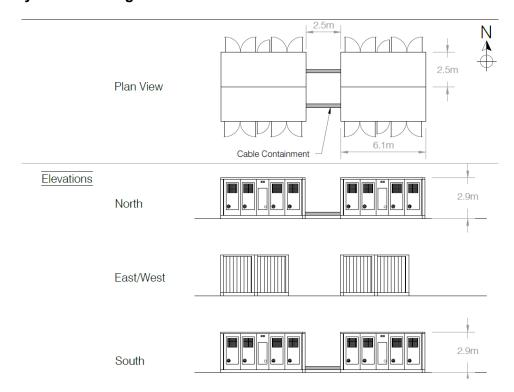
A cluster would comprise four batteries, with a total of 24 BESS battery clusters being provided.
